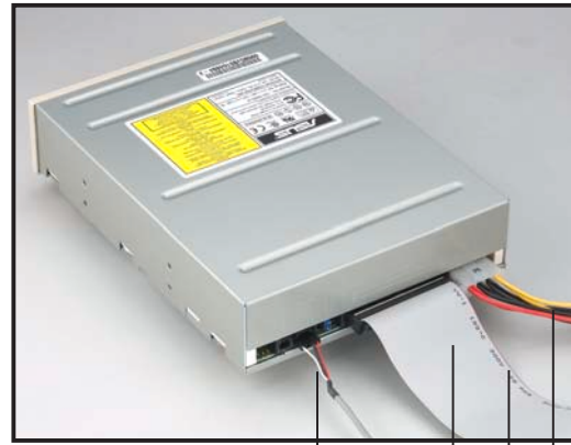
CD-ROM audio cable IDE ribbon cable Red stripe to Pin 1 Power cable (P1)
